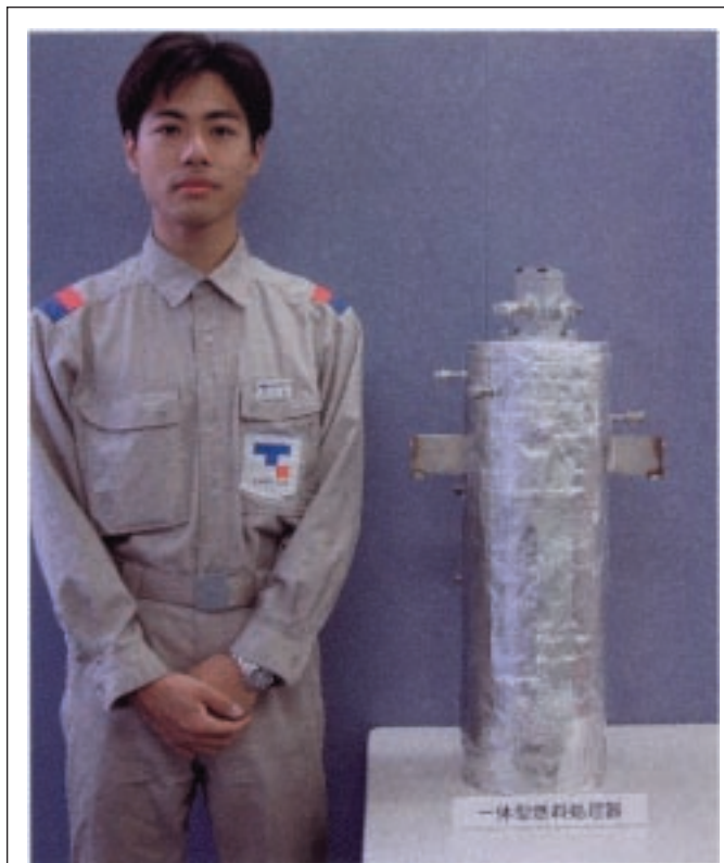
Figure 3. 1 kW fuel cell incorporating hydrogen generation system.
